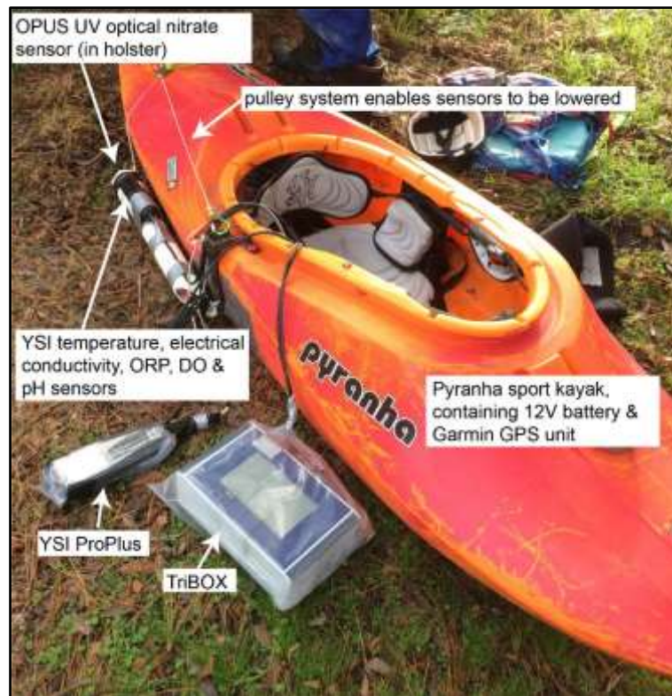
Figure 2. Instrument set-up on white-water kayak used for stream surveys.
