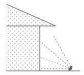
Select fixture beam spread and orientation, to minimise projection beyond target area
