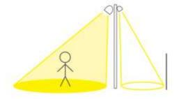
Select output intensity and beam spread to avoid excessive brightness or unnecessary coverage
