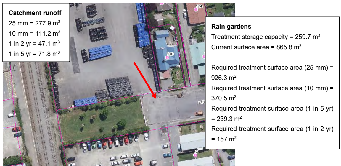
Figure 7. Keir Street pipe manufacturers yard rain garden
