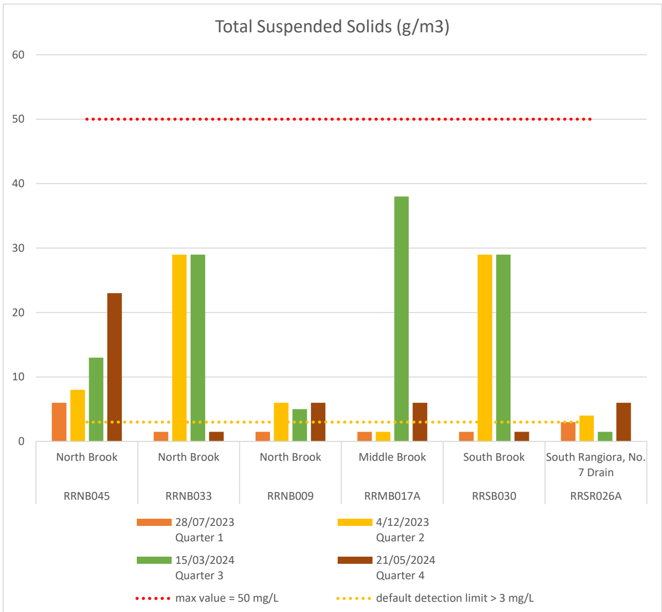
Figure 12. Total suspended solids for Major Network Outlets sampling FY 23/24. Values below the default detection limit, are represented as half the detection limit (1.5 mg/L).
