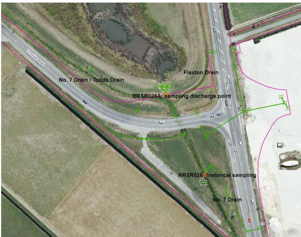
Figure 14. Discharge sampling points and baseline (historical sampling) sites shown in relationship to Pond C and the receiving environment.
