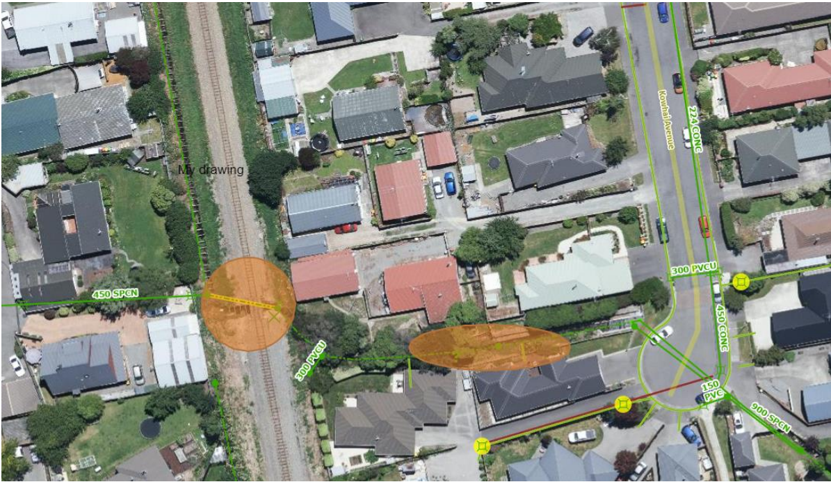
Figure 22. Kowhai Ave: Suggested area for stormwater improvements to address dissolved copper exceedances in the north book higher up the catchment (RRNB033). Note: there is another project underway looking at addressing these exceedances upstream. They are also addressed further down the catchment with North Brook Ponds, with recorded reduced levels of dissolved Copper.
