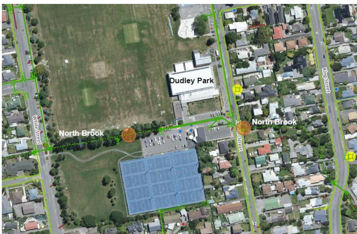
Figure 21. Dudley Park: Proposed area for stormwater improvements to address dissolved copper exceedances in the North Brook higher up the catchment (RRNB044). Note: these exceedances are currently addressed further down the catchment with North Brook Ponds, with recorded reduced levels of dissolved Copper.
