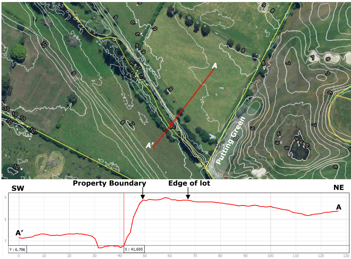
Figure 3: Topography of the southern end of the site, with 0.5m contours (above image). Cross section showing the elevation difference stream and the site above (below image).
