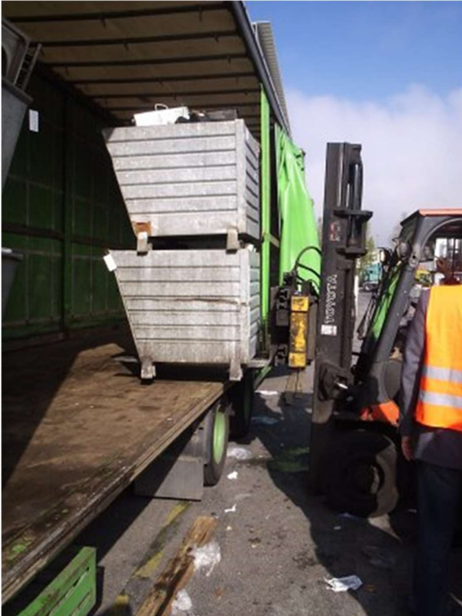
Figure 22: Standardised Bins Being Loaded onto Curtainsider Truck
