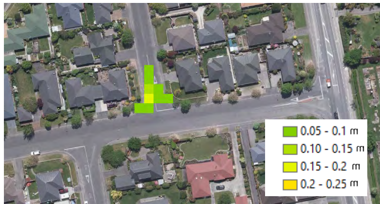
Figure 3. Modelling of Option 2 configuration during 1 in 5 year one hour storm
