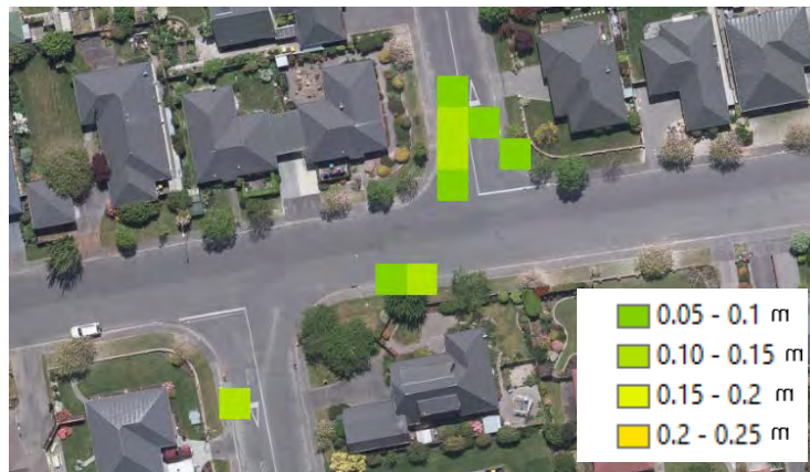
Figure 4. Modelling of Option 4 configuration during 1 in 5 year one hour storm
