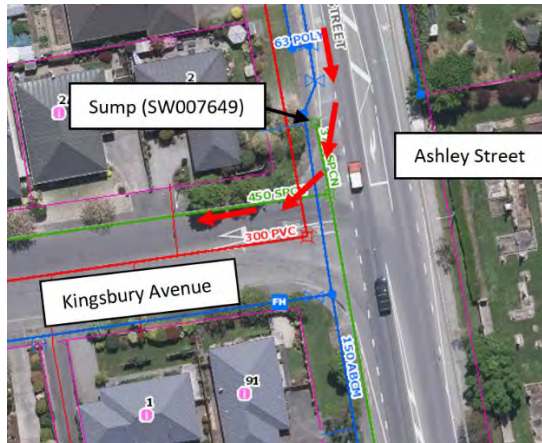
Figure 2. Flow from upper Ashley Street to Kingsbury Avenue
