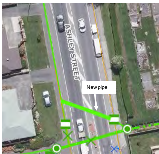
Figure 5. New pipe across Ashley Street
