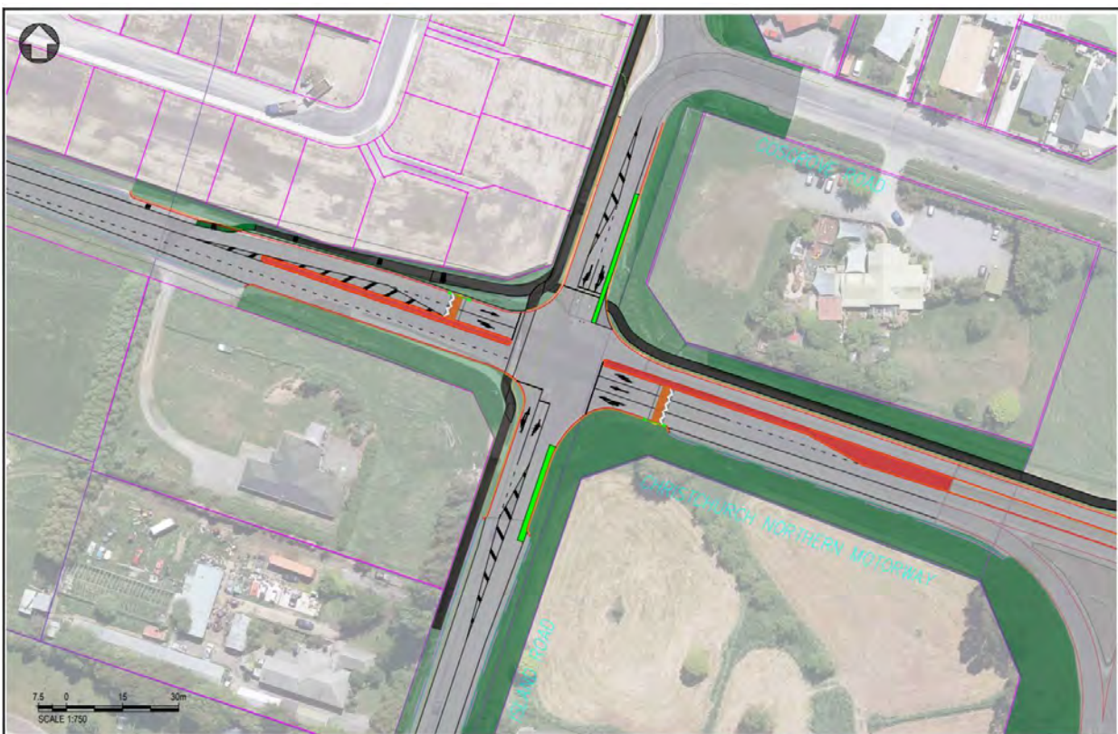
Figure 14 Traffic signals option scheme design (WDC design)
