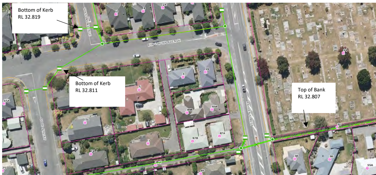
Figure 6: Bottom of kerb elevations compared to bank height of the cemetery drain.
