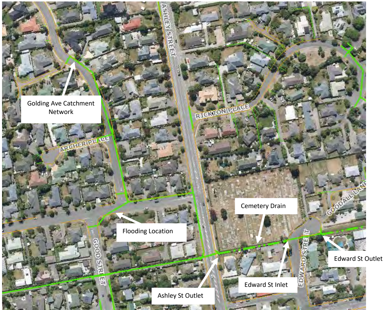
Figure 1: Aerial of Golding Ave stormwater network catchment
