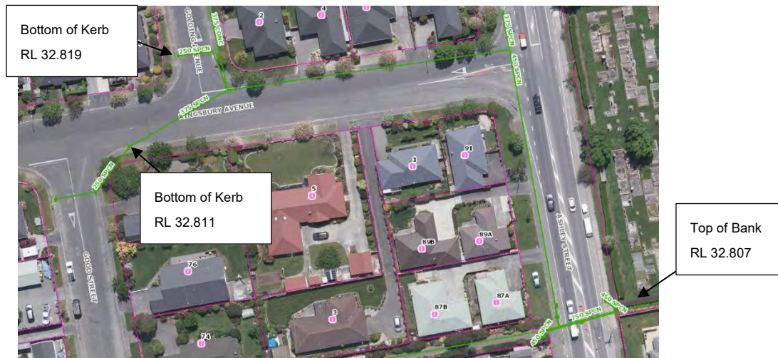
Figure 3. Elevation comparison of cemetery drain and low points upstream
