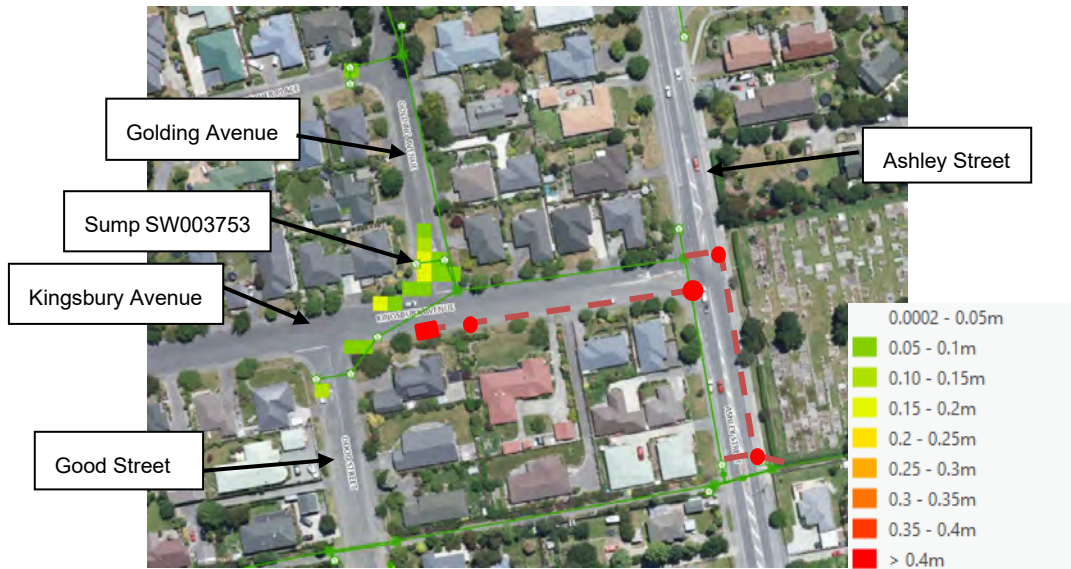
Figure 5. Flood modelling results on the capacity upgrade option (red lines indicate new pipe) at Kingsbury Avenue
