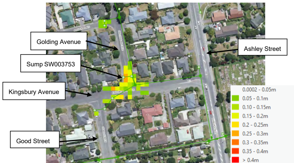
Figure 3. Flood modelling of the upgraded sumps at Golding Avenue, Good Street and Kingsbury Avenue
