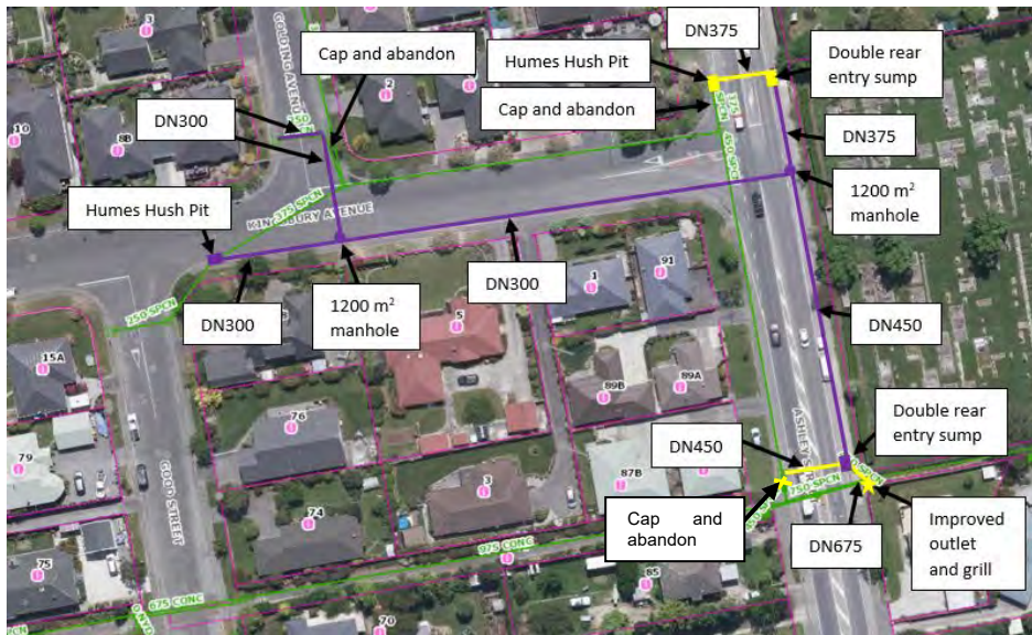
Figure 1. Recommended two stage approach to stormwater upgrades
