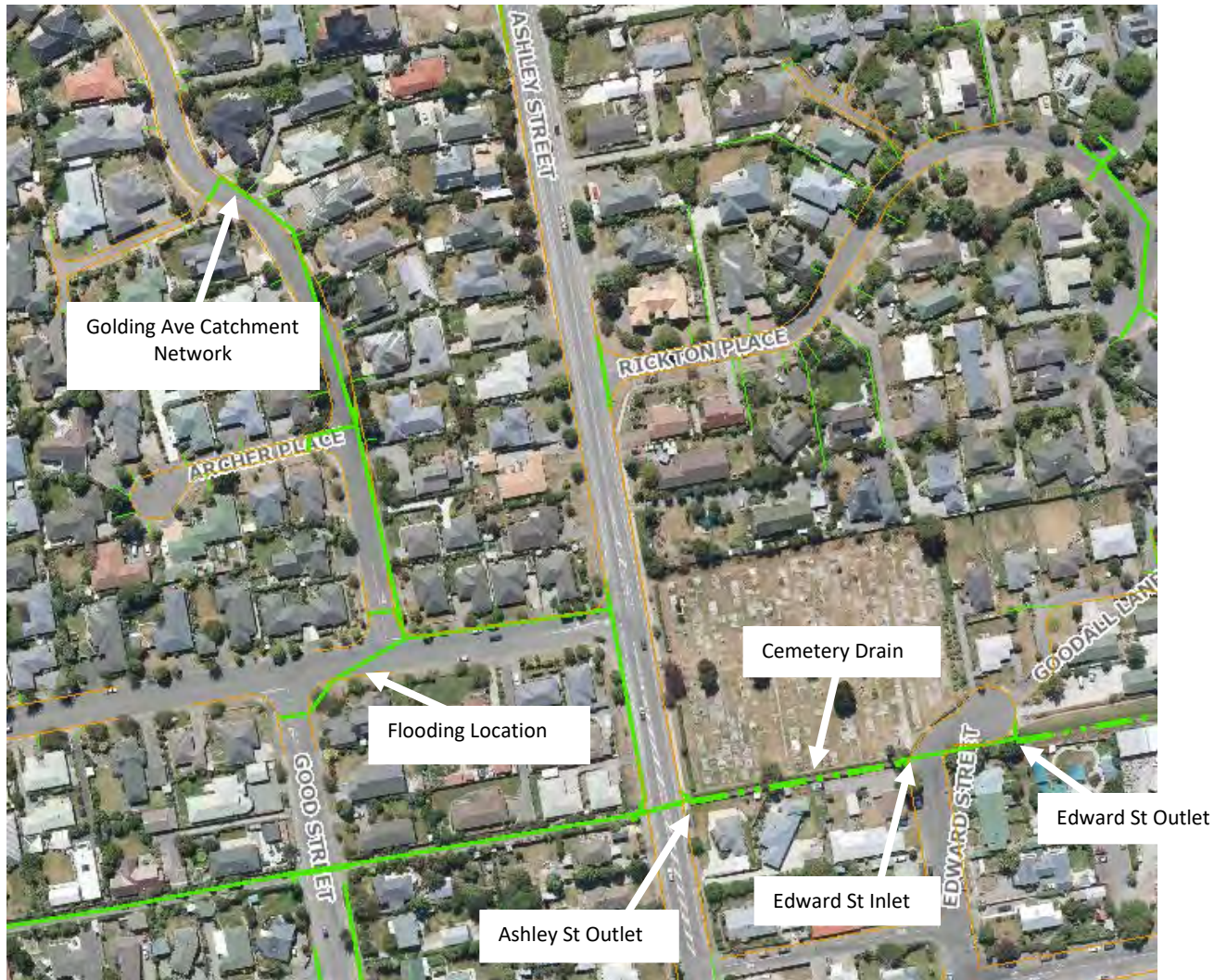
Figure 1: Aerial of Golding Ave stormwater network catchment
