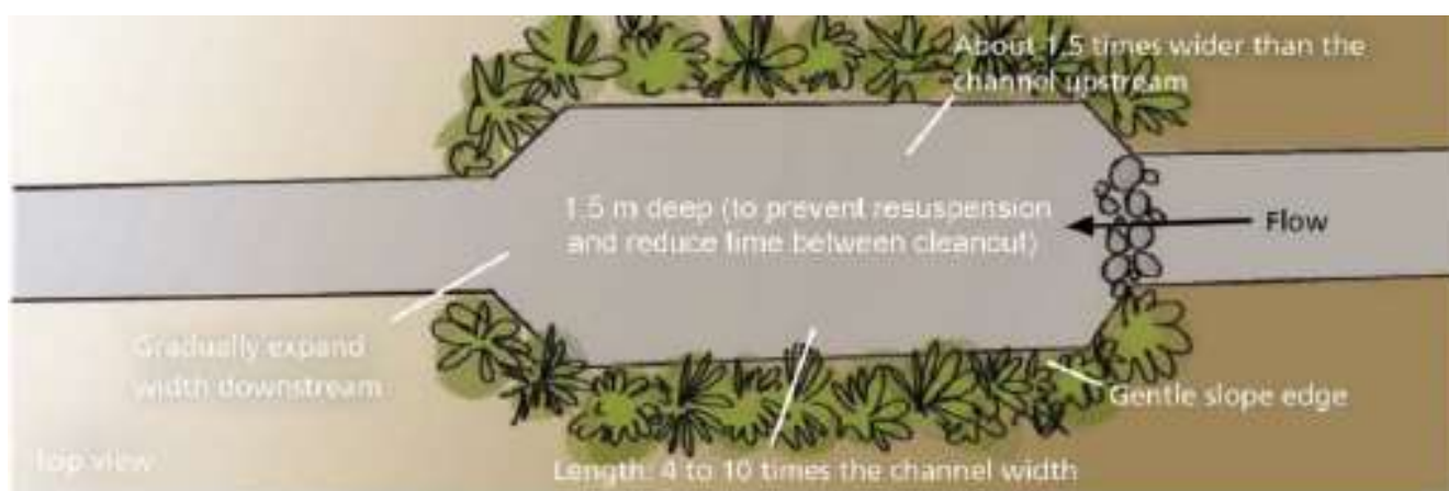
Figure 13: Sediment Trap Design
