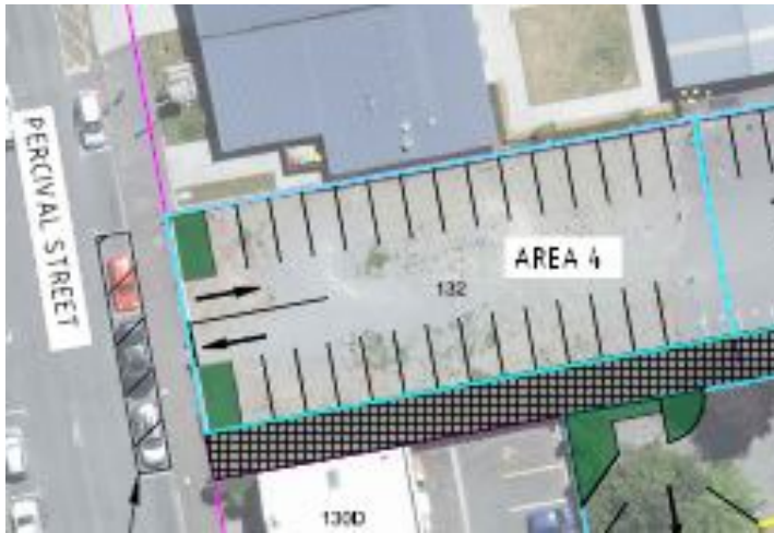
Figure 2 – 132 Percival Street temporary carpark design example NB: the Percival Street entrance will not be available in the final constructed carpark. The carpark will contain wheel stops only and not wooden parking bay demarcation barriers.
