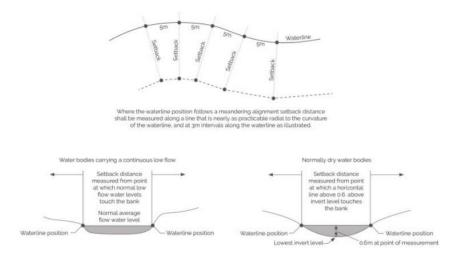
Setback distance measured from point at which normal low flow water levels touch the bed.
