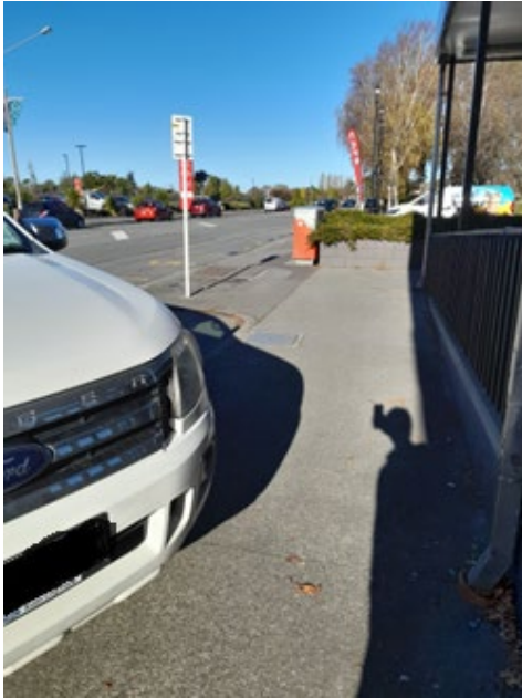
Photograph 1: Vehicle over-hang over the footpath associated with the current angle-parking layout.
