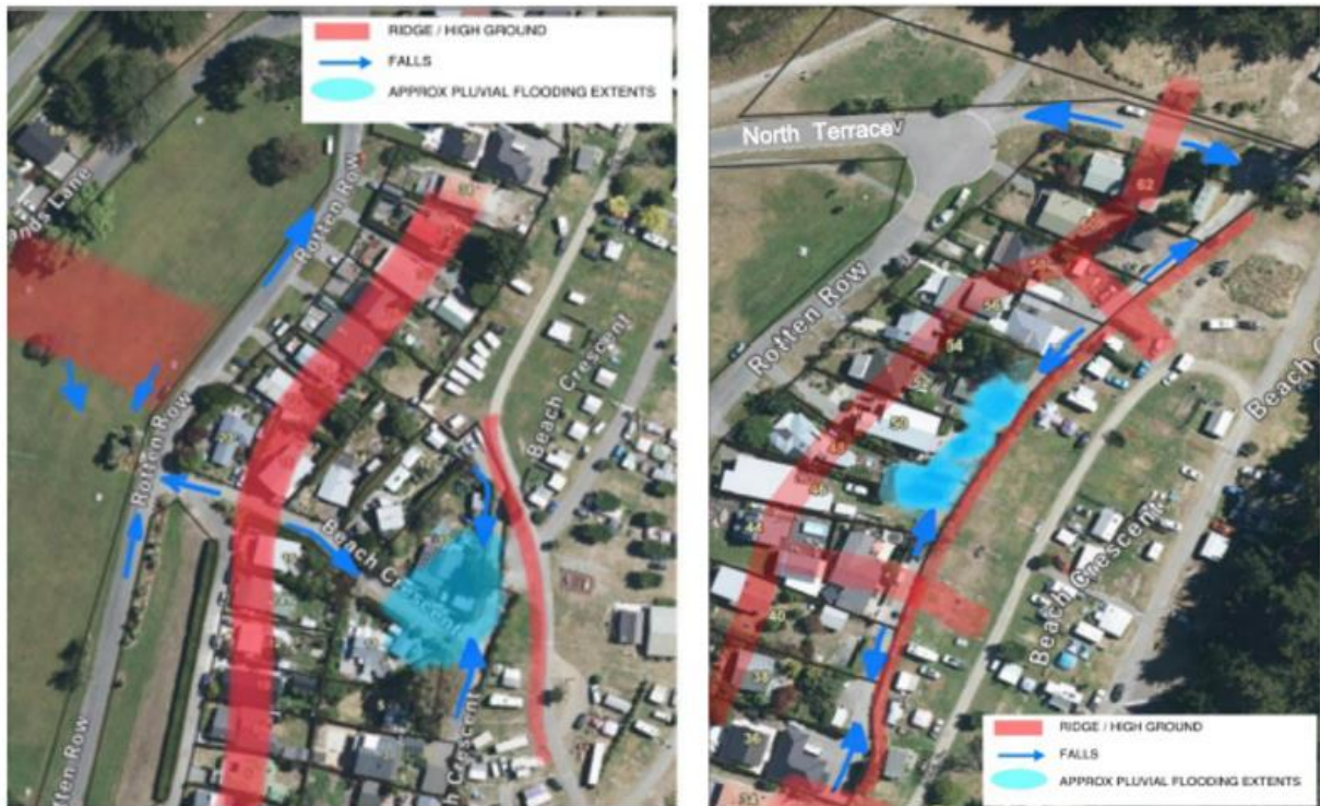
Figure 2 - Flooding Extents: Beach Crescent (left) Rotten Row (right)
