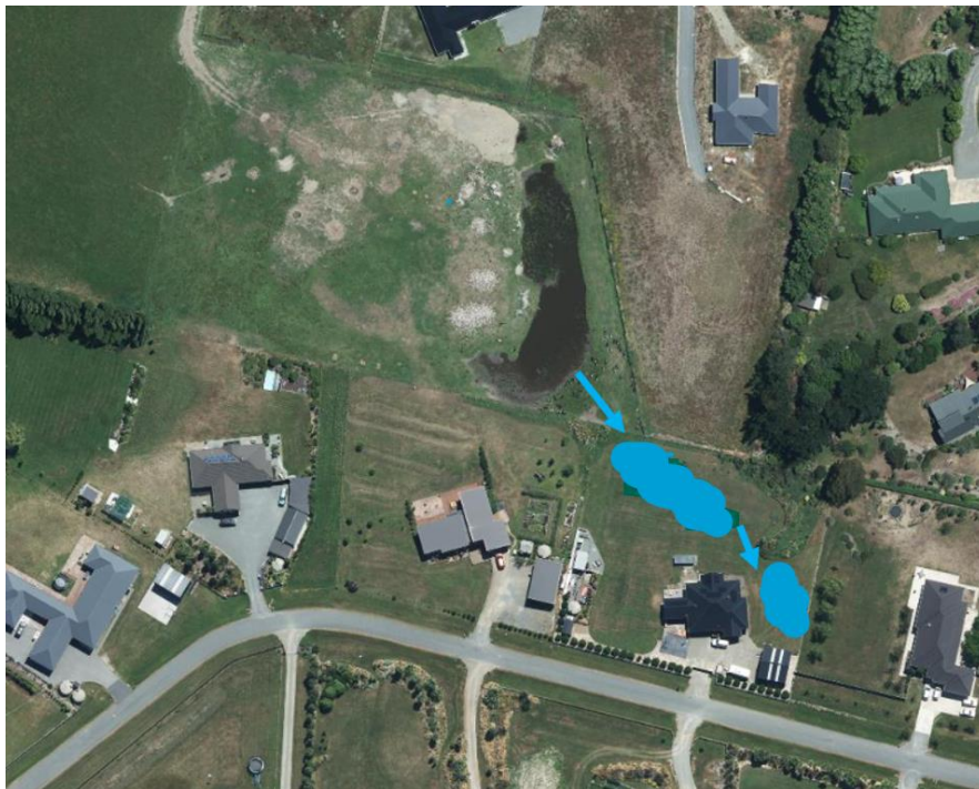
Figure 11 - Pond Overflow Path
