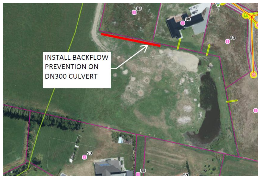
Figure 13 - Culvert back-flow prevention install
