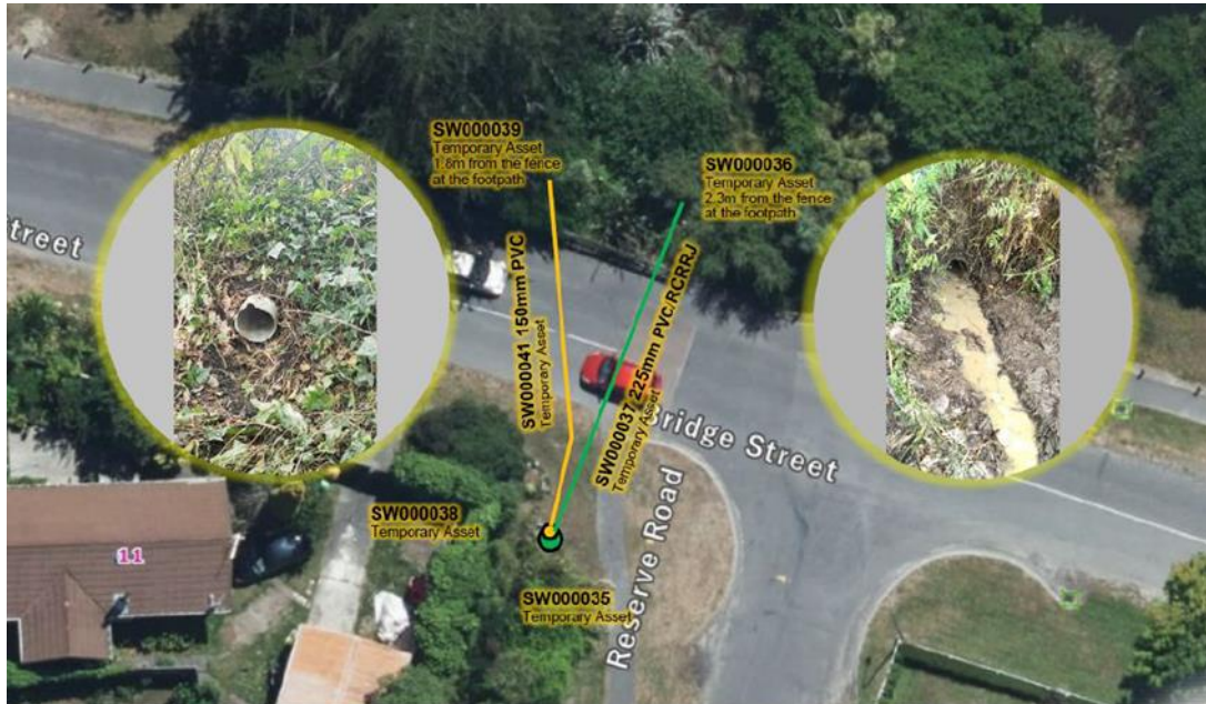
Figure 7 - CCTV report pipe locations and outlets
