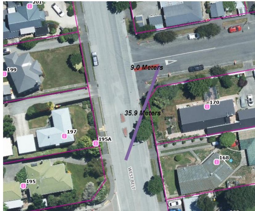
Figure 5. Available sight distance at the intersection of Seddon Street and West Belt.
