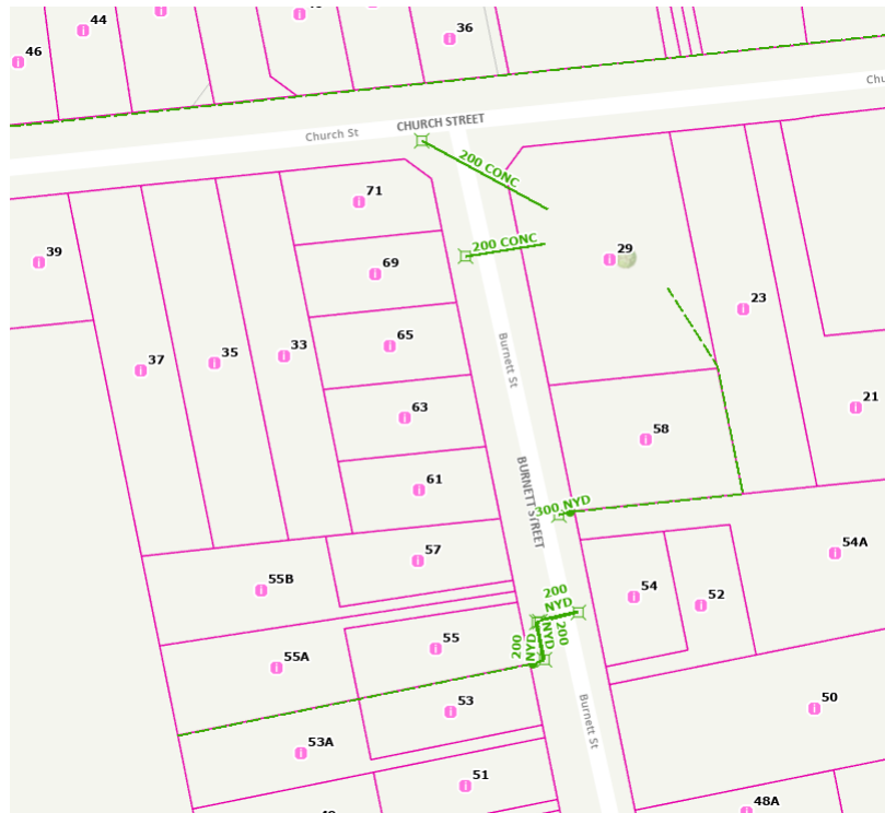
Figure 11: Existing Stormwater Layout: 51 – 71 Burnett Street
