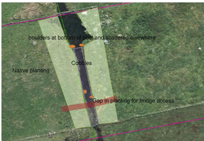
Figure 3: Restoration at 428 Tuahiwi Road. The light green indicates native planting. A few boulders and some cobbles will be added to improve in-stream habitat.
