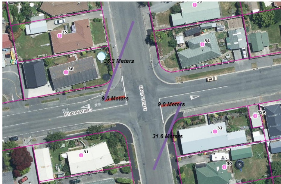
Figure 3. Available sight distance at the intersection of Seddon Street and Kinley Street.
