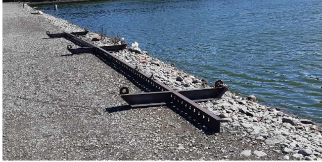
Figure 1: The dredge that has been designed by 3 Waters staff for use at Kaiapoi WWTP, and nicknamed the ‘the Midge-buster’
