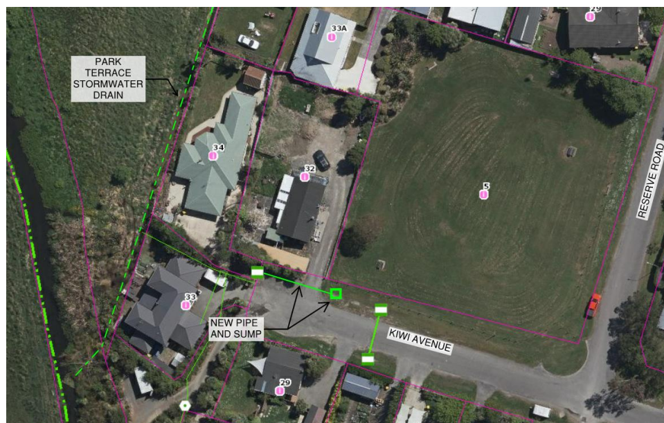
Figure 5. Kiwi Avenue drainage works.
