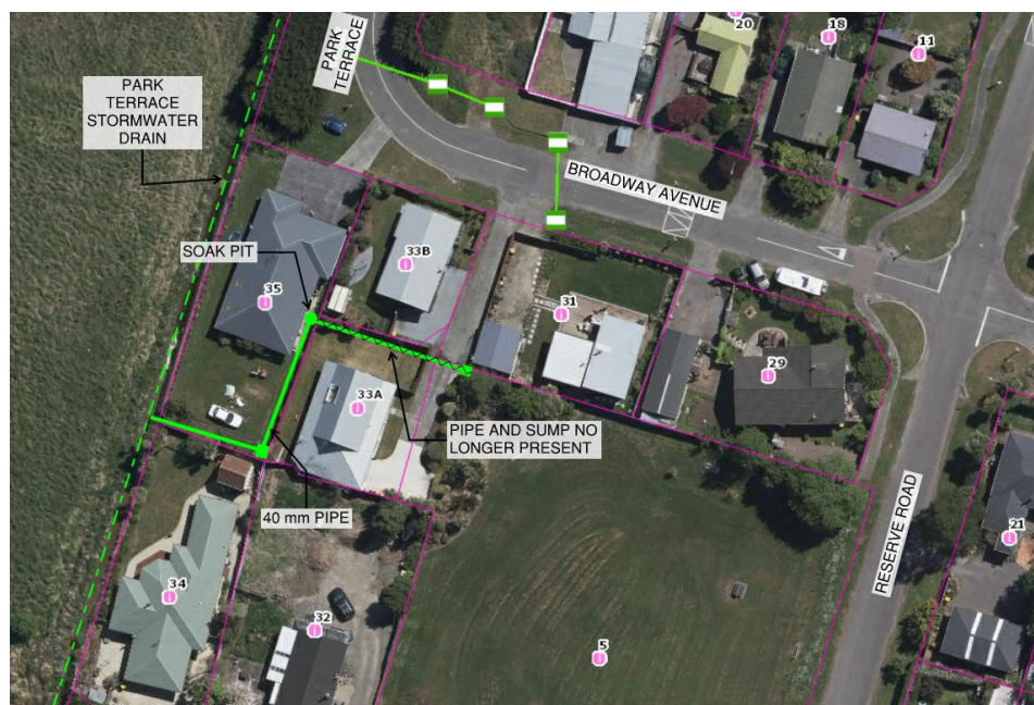
Figure 4. 35 Broadway Avenue stormwater pipes.
