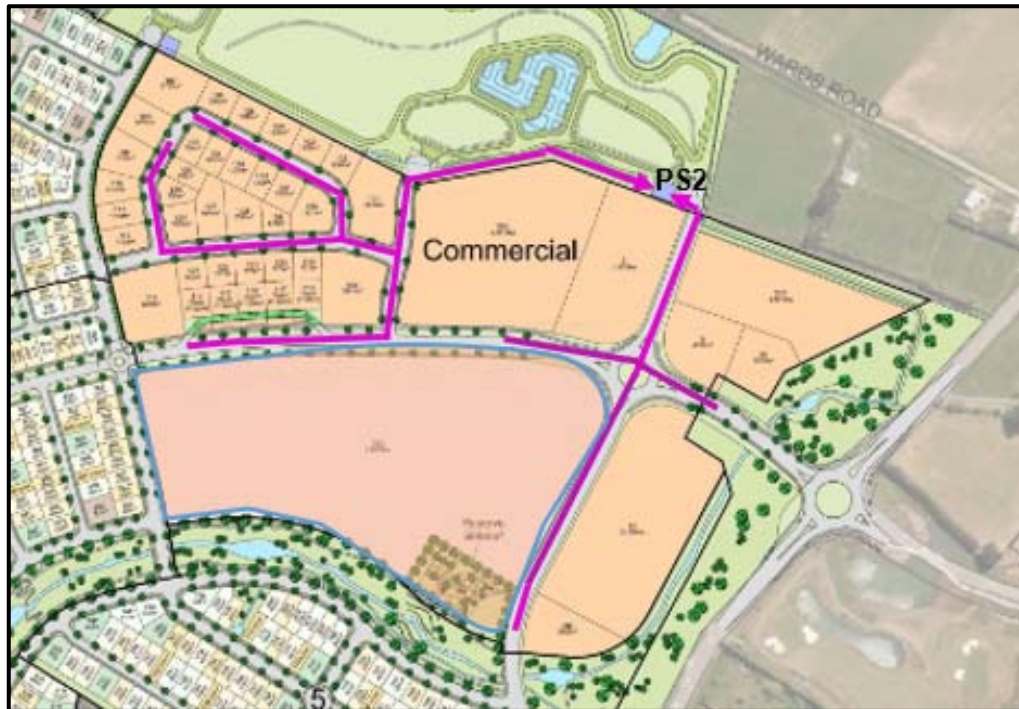
Figure 3: Indicative sewer alignment
