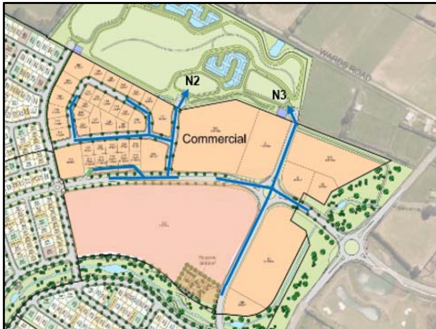
Figure 6: Indicative Primary Stormwater Network Layout
