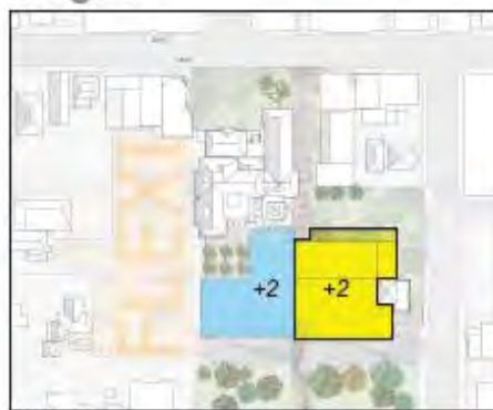
New Library & RSC South Wing (Decant library to new build, RSC 2/lvs) RSC: 5360m 2 Library: 2980m 2 Total GFA: 8340m 2
