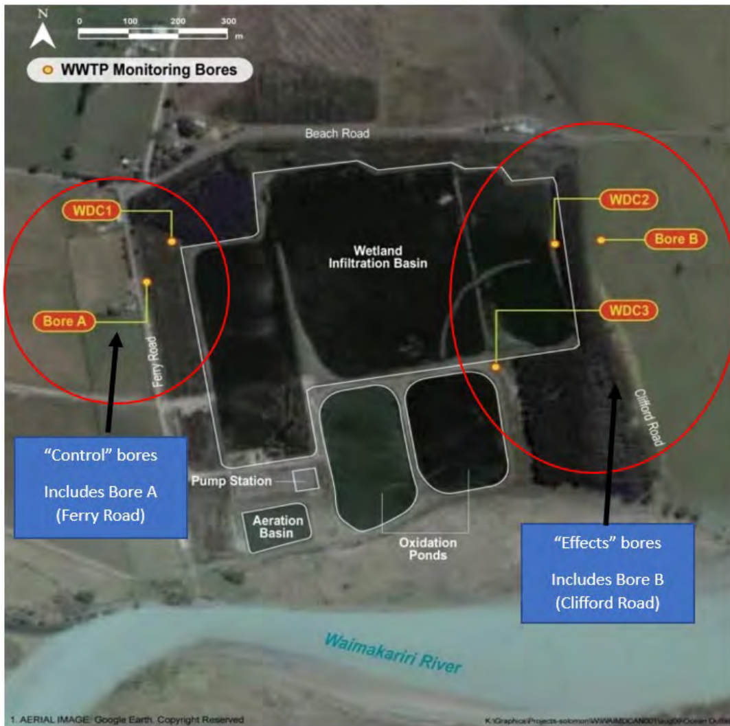
Figure 24: Location of Kaiapoi monitoring bores
