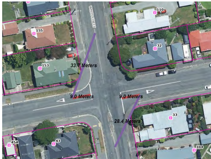
Figure 2. Available sight distance at the intersection of Seddon Street and White Street.
