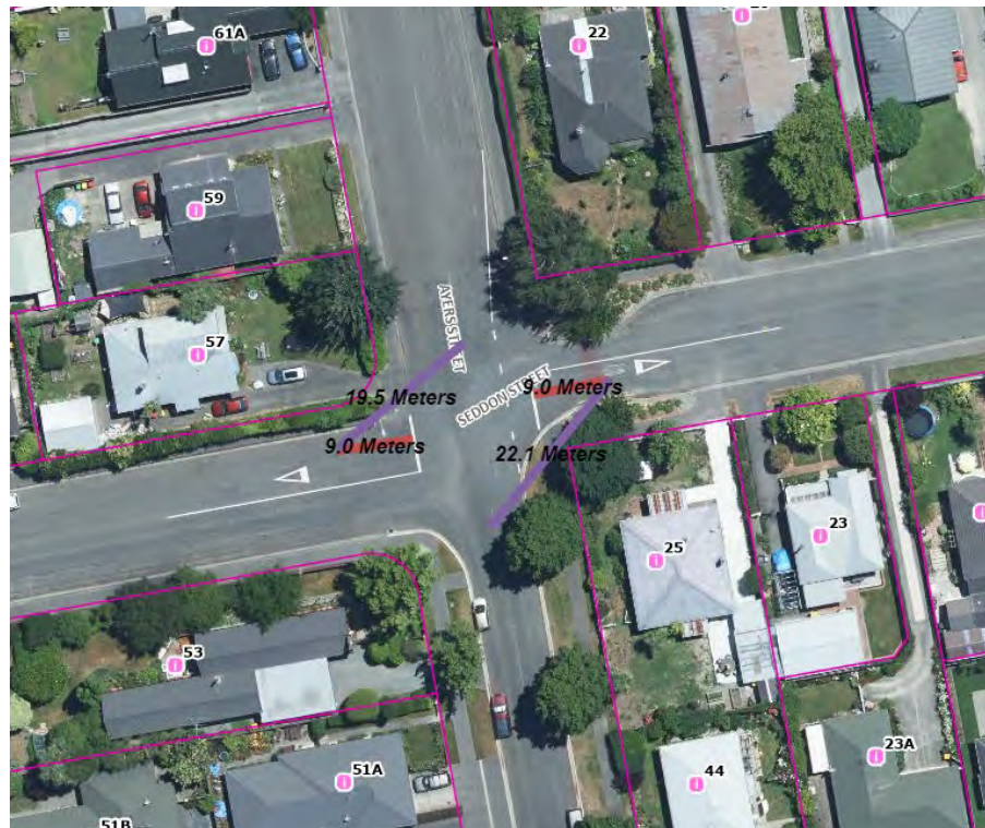
Figure 1. Available sight distance at the intersection of Seddon Street and Ayers Street.
