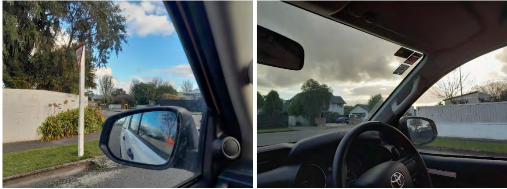
Figure 14. Visual of sight distance available at the Seddon Street/West Belt intersection on the eastern approach.
