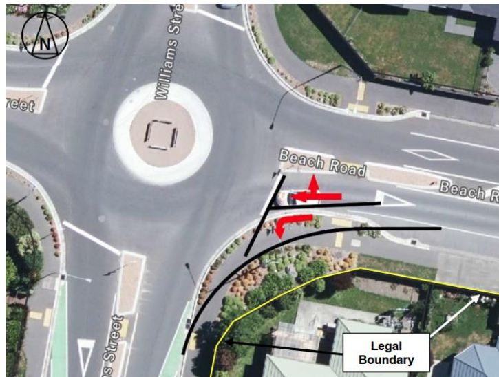
Figure 7: Evidence of Mr Carr, Appendix A, Figure 16: concept second lane to accommodate 'low' development scenario traffic
