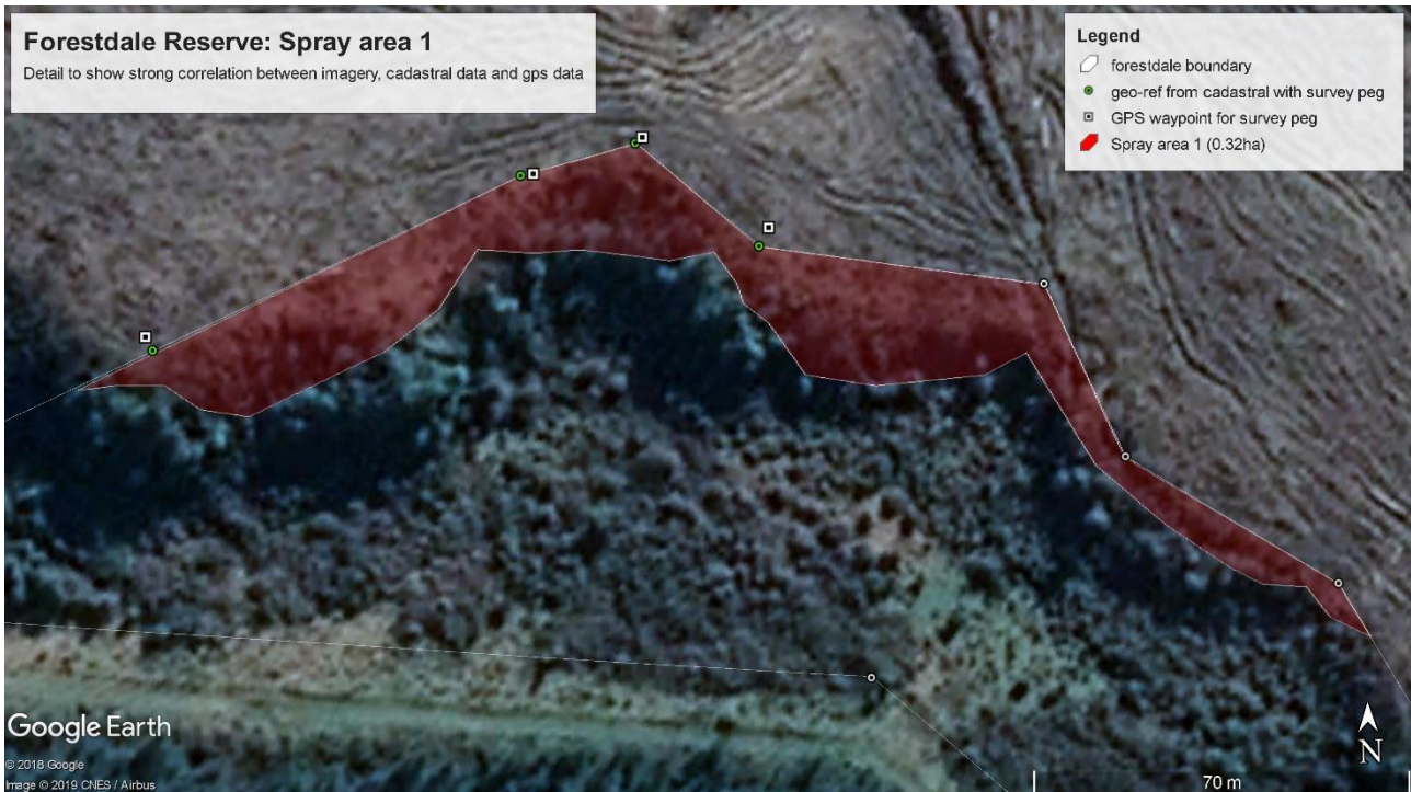
Figure 4 Close up of spray area 1 to demonstrate reliability of the cadastral overlay
