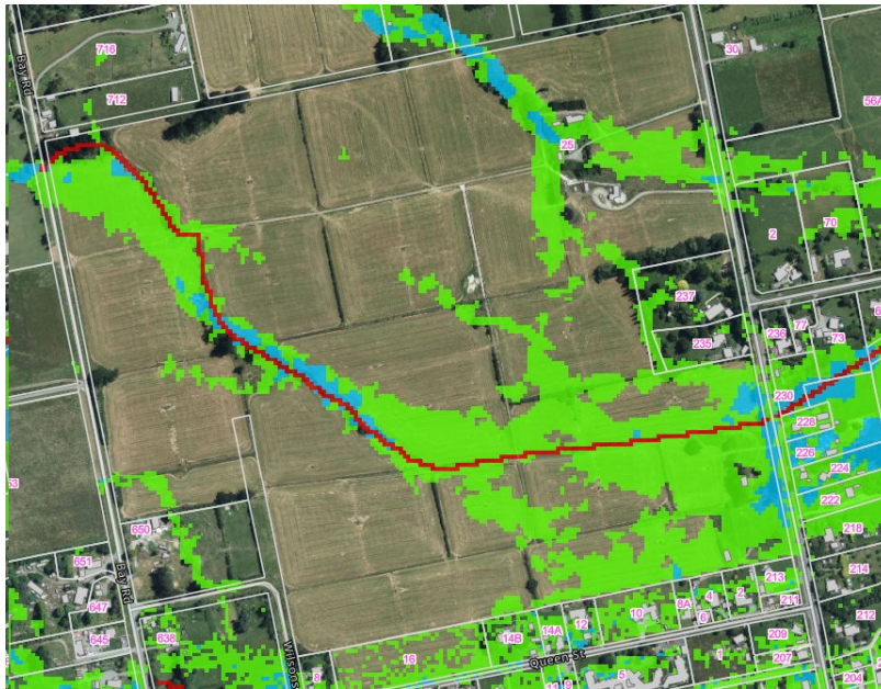
Figure 43: Flooding and stormwater flow path for 25 Ashley Gorge, Oxford
