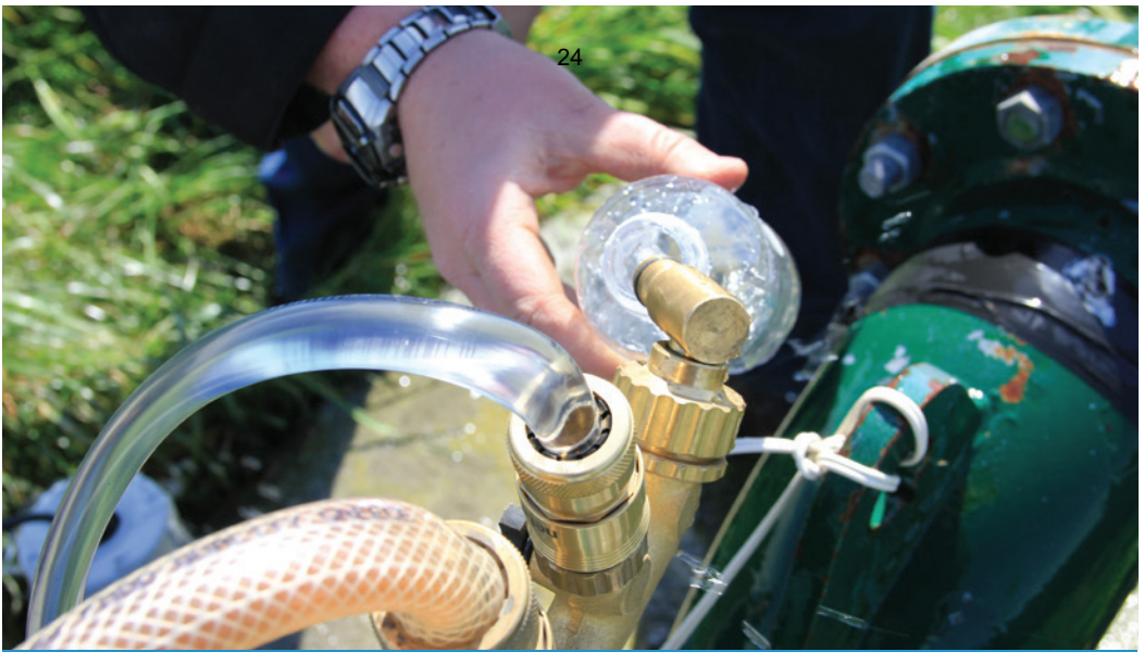
Taking a water sample at a wellhead
