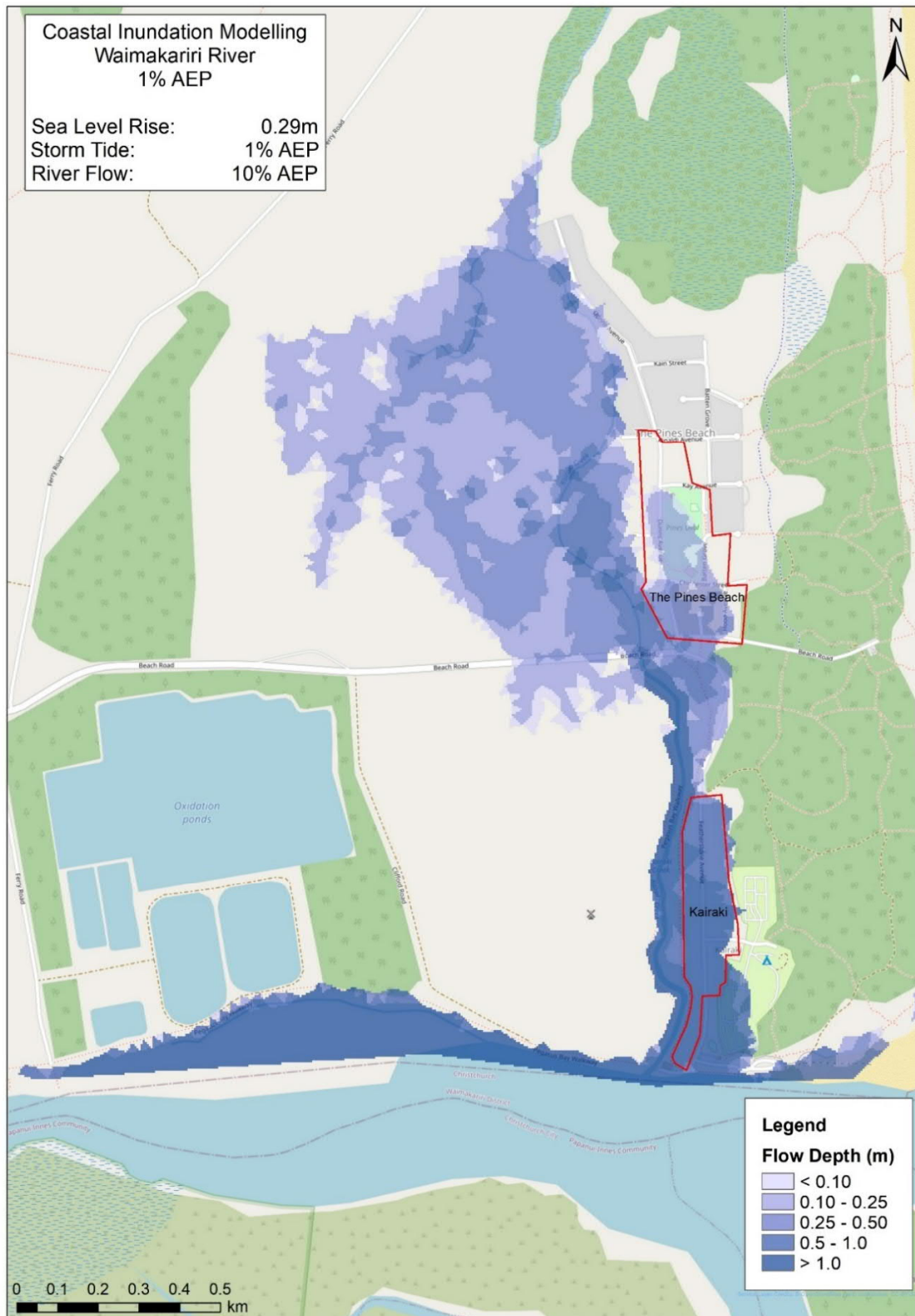
Figure 5 Model flood extent for 1% AEP storm tide and 0.29 m rise in mean sea level with design stopbank levels
