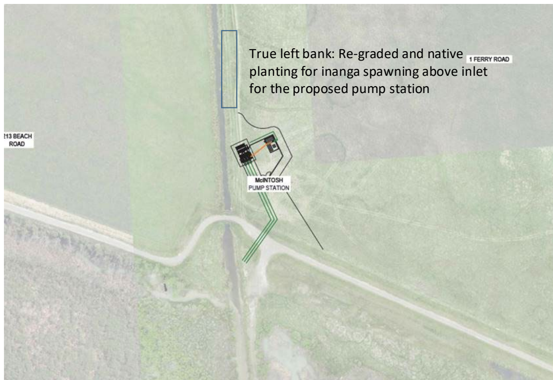
Figure 4: The location of the proposed bank re-grading, followed by native planting on the McIntosh Drain, north of a newly-commissioned pump station.
