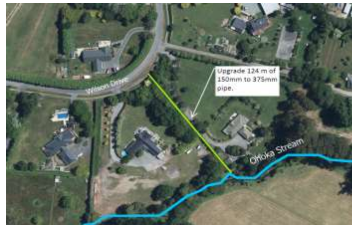
Wilson Drive Stormwater Improvements
