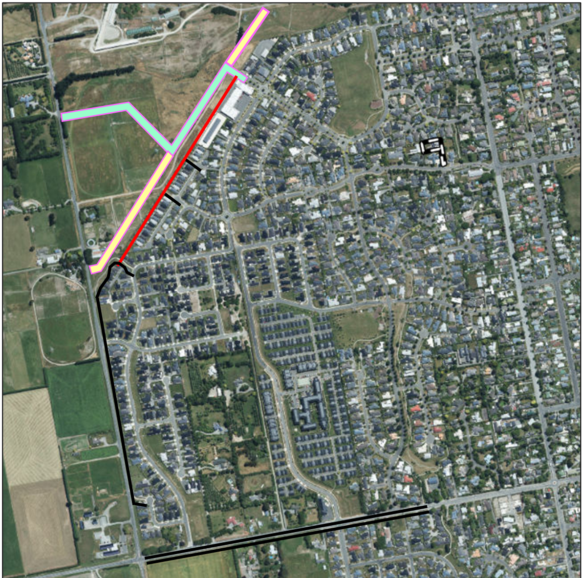
Figure SE3: Existing marked cycleway network in the vicinity of the subject site (shown in black) with the recommended shared path addition shown in red.
