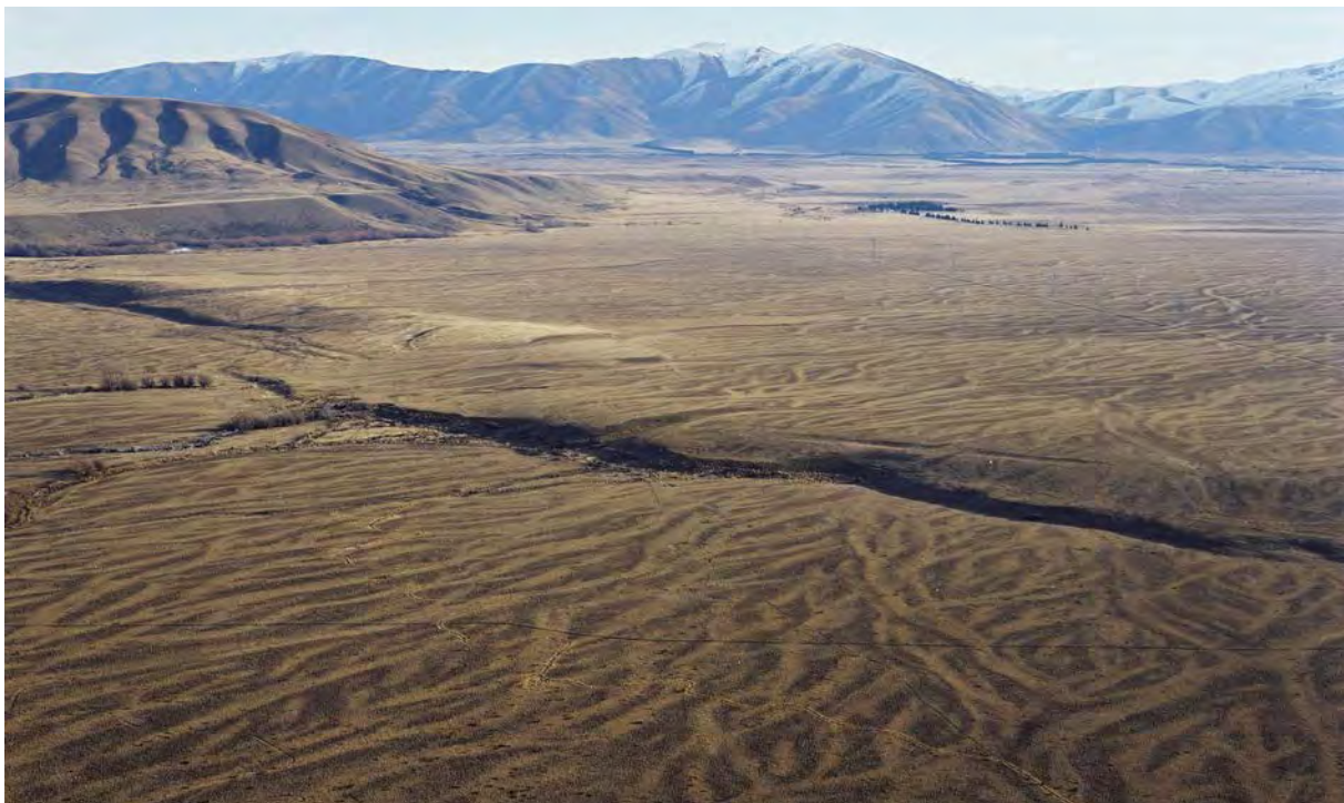
Figure 2.2 The Ostler Fault Zone, in the Waitaki and Mackenzie districts, runs from upper left to lower right, and has offset and buckled old braided river channels. At the far left, the fault scarp (in shadow) is sharply expressed. Heading towards the photo centre, the fault scarp evolves into a broad fold which flattens out near the photo centre. At that point, another fault scarp and associated fold has emerged 200 m or so in front of it, and continues towards the right. This view shows an array of faults and folds which all form part of a single entity, the Ostler Fault Zone. Photo: GNS Science; D.L. Homer, catalogue number 3418/2 H, taken July 1982.
